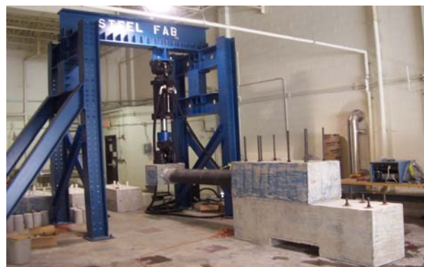
Figure 11. Test Set-up for Long Carbon Tube.
