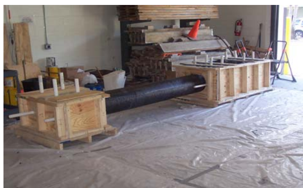
Figure 9. Preparation of Long Carbon Specimen.
